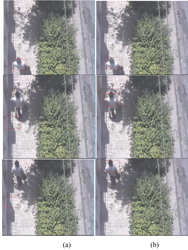
Figure 2. Tracking a pedestrian without kernel modification (a) and with kernel modification (b).
