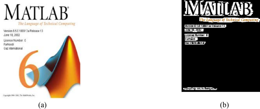
Figure 5. A sample image to illustrate the robustness of the proposed algorithm against font size. (a) Original image, (b) extracted text regions.
